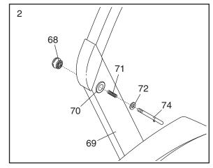
With the help of a second person, carefully tip the Uprights (69) down as shown. Make sure that the Extension Legs (102) remain in the Uprights.
